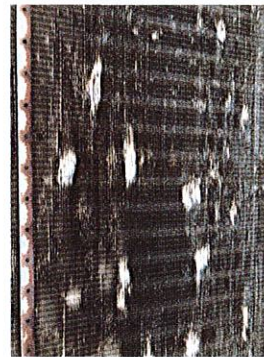
Condenser fin damage
